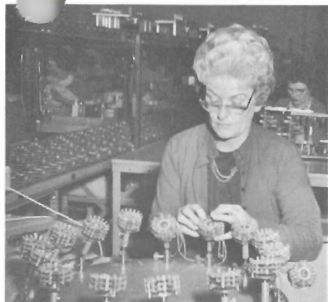
Careful attention to wiring attenuator switches for amplifiers is given by Eleanore Dobbins.
