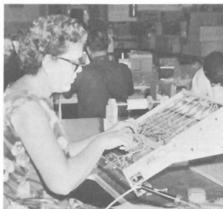
Amplifier in 8-channel recording system is wired by Evelyn Bright. Uses are both medical, industrial.
