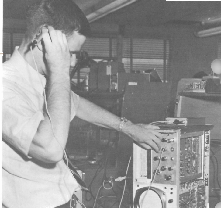
John Hart, engineering, uses his head to run check on newly developed ultrasonic A-scan unit. Instrument will make important contribution to medical technology.
